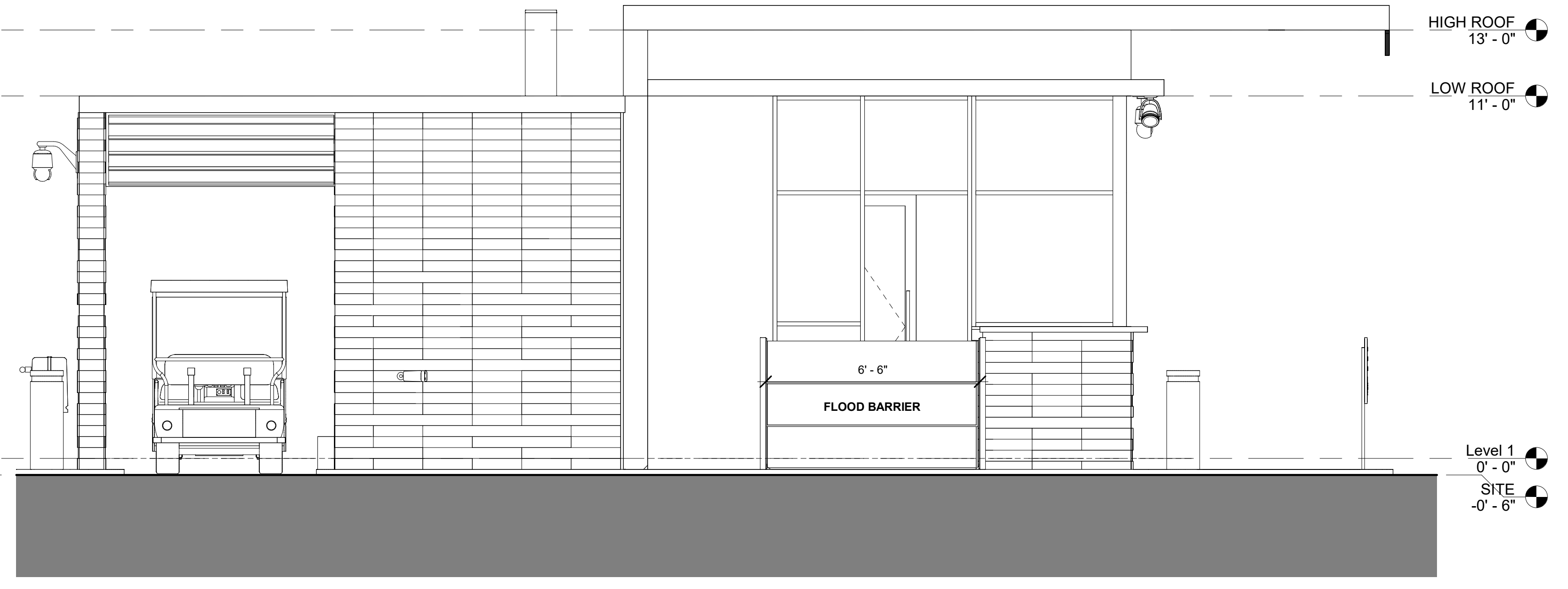
2 P-3 PROPOSED EAST ELEVATION - WITH FLOOD BARRIERS 3/8" = 1'-0"
